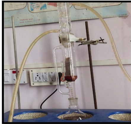
Fig 1: Extraction of Hibiscus by Soxhlet Extraction
