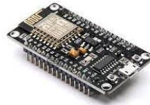
Fig.6. NodeMCU ESP8266 microcontroller with Wi-Fi module
