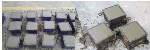
Fig :- Casting of cube
