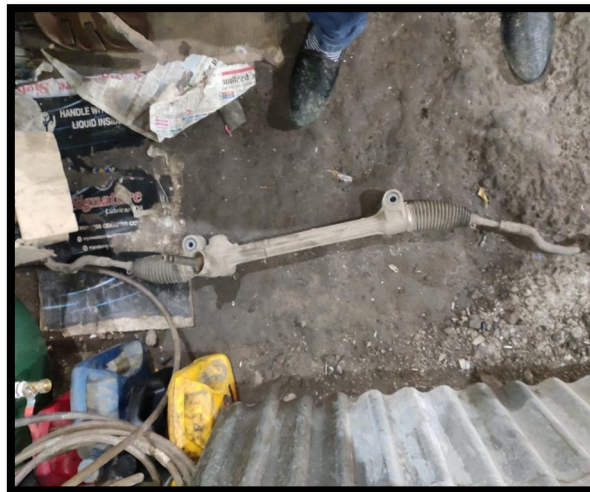
Fig 1 - Old rack and pinion steering
