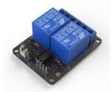
A relay is an electrically operated switch. It consists of a set of input terminals for a single or multiple control signals, and a set of operating contact terminals. The switch may have any number of contacts in multiple contact forms, such as make contacts, break contacts, or combinations thereof.
