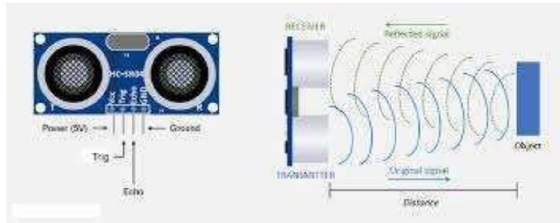
Figure 2: HC-SR04 Ultrasonic Sensor Working
