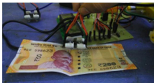
Figure 6: Note calibration by one colour sensor
