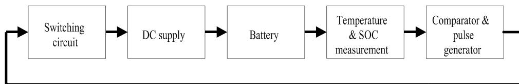
A block diagram of the control strategy of temperature-regulated pulse charging is shown in above Figure .The first block is switching circuit. It has two main functions, firstly it disconnect the dc supply when battery temperature goes beyond the pre-set limits which are maximum and minimum temperature limit and secondly it break the supply when SOC percentage of battery goes up to 95 percentage. Second block is DC supply block. To charge the battery at higher rate, higher voltage
