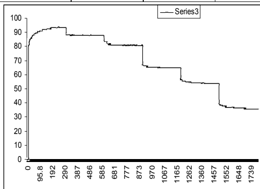
Extension verses Time curve of 70 Denier Yarn.
