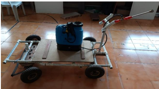
Fig .3 Structure building, sprayer integration Electrical connections and wireless manual testing
