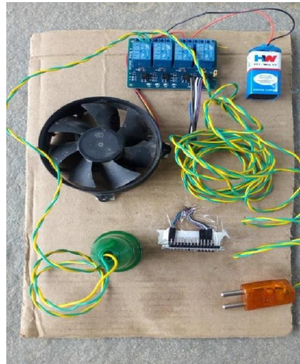
Fig: Connections of Google Assistant-controlled Home automation
