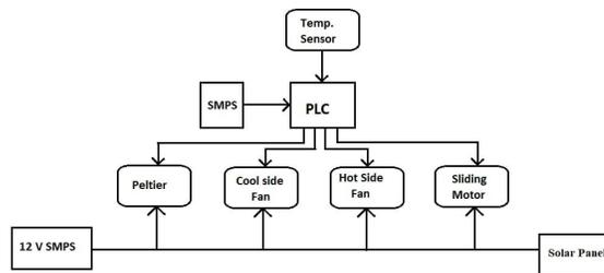
In the block diagram a separate SMPS module is shown which is used to run PLC. Next temperature sensor is used which will sense the temperature. Next 12V SMPS module is used to give supply to peltier module, cooling fan ,heating fan and sliding motor. The peltier module will produce cool as well as hot air so here we are going to utilize both the air for different purposes. Cold air will preserve the air for long time and hot air will use for drying the dry fruits and other produce.
