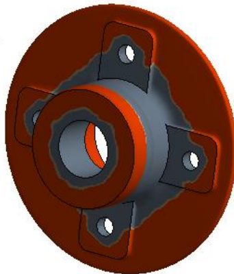
Fig. Topology optimization results
