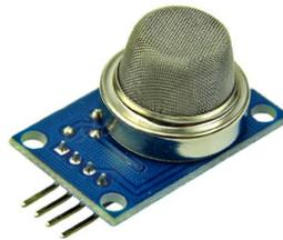
This is a simple-to-use MQ-6 Liquefied Petroleum, iso-butane, propane gas Sensor module, suitable for sensing LPG (composed of mostly propane and butane) concentrations in the air. The MQ-6 can detect gas concentrations anywhere from 200 to 10000ppm. This sensor has a high sensitivity and fast response time.
