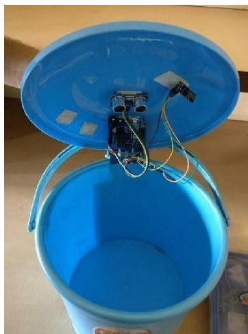
Figure 2: Bin with Level sensor
