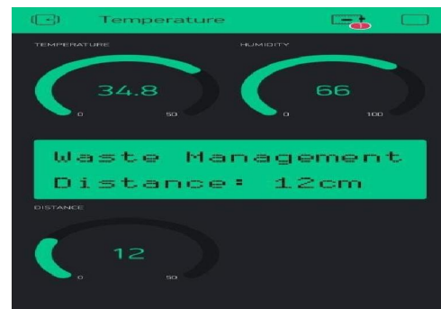
Figure 3: Blynk output of Level sensor
