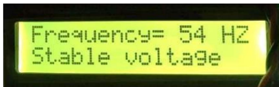
Fig. 2. High frequency condition
