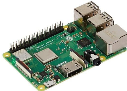
Fig.1. Raspberry Pi 3b
