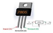
A voltage regulator is a component of the power supply unit that ensures a steady constant voltage supply through all operation conditions. It regulates voltage during power fluctuations and variations in loads. It cant regulate AC as well as DC voltages.
