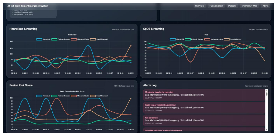
Figure 3. Caregiver dashboard streaming panels: real-time heart-rate and SpO2 trends per patient, the fusion risk-score trend (screenshot of live prototype) and the rule-based alerts log.
