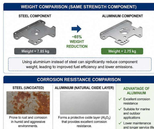
Figure 7: Comparison of aluminium and steel highlighting the advantages of aluminium in terms of weight reduction and corrosion resistance
