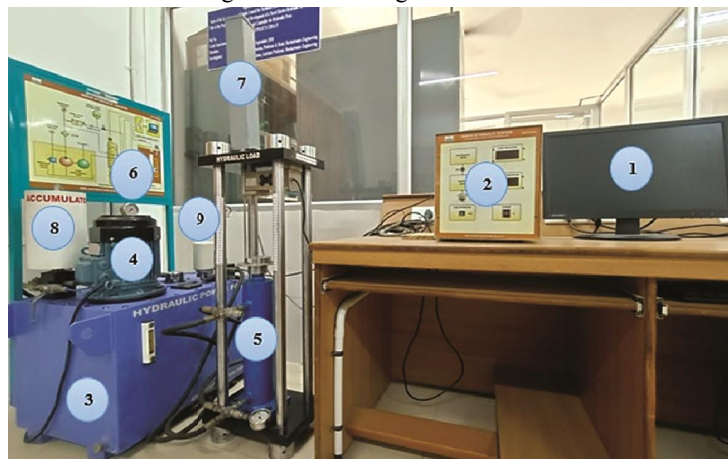
Fig. 2:Photography of EHSS: 1-Personal computer (PC), 2-DAQ, 3-Hydraulic power pack, 4-Three phase fixed displacement pump, 5-Double-acting hydraulic cylinder, 6-Pressure gauge,7-LVDT, 8-Accumulator, 9-Servo spool valve
