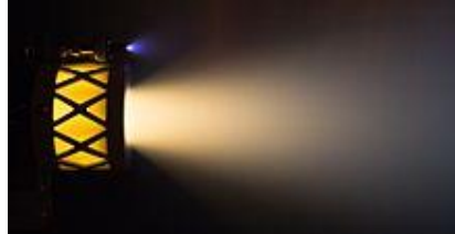
Figure 1.10 Busek's BIT-3 ion thruster proposed for NASA's Lunar IceCube mission
