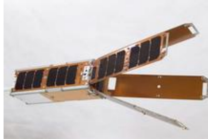
Figure 1.11 Winglet solar panels increase surface area for power generation
