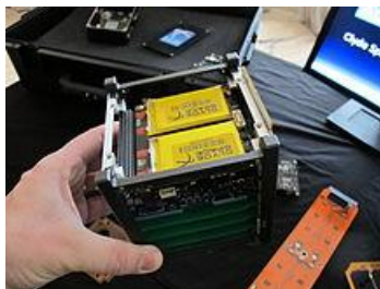
Figure 1.7 1U CubeSat structure
