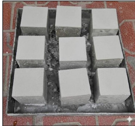
Fig 4: Concrete Test Cubes
