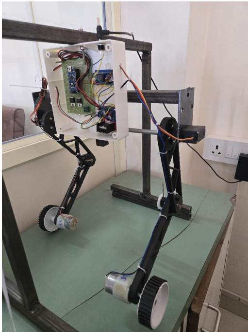
Fig. 7. Full prototype robot during load testing and gait simulation showing both leg assemblies, the electronics enclosure, and the steel
