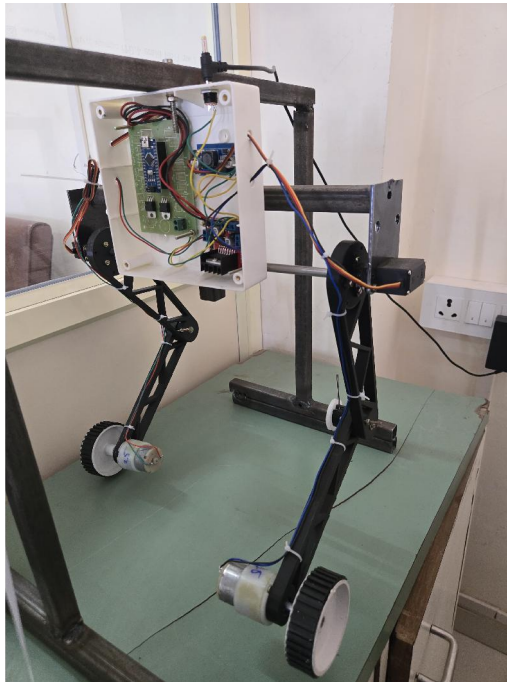
Fig. 1. Physical prototype showing the overall system architecture, chassis frame, microcontroller enclosure, and dual leg assemblies.
