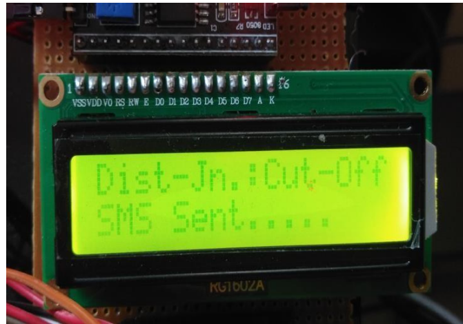
Figure 4.5: Automatic power cut-off message display
