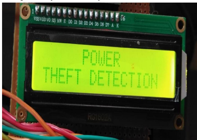
Figure 4.4: Power theft detection message display(LCD)
