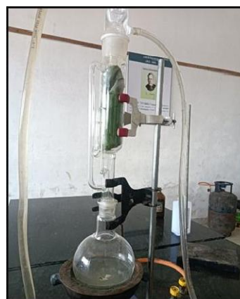
Figure no.3: Leaf soxhlet extraction Albizia saman IV. QUALITATIVE PHYTOCHEMICAL ANALYSIS
