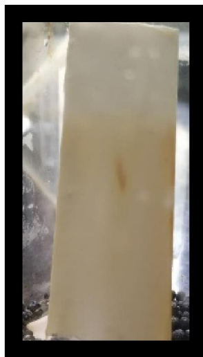
Fig no. 08: TLC plate showing spot with Rf value of 0.69
