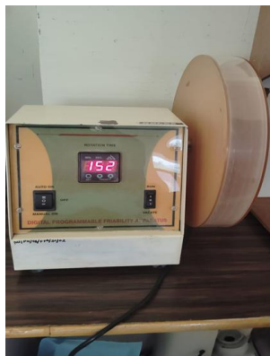
Figure 2: Digital programmable friability apparatus (Roche-type) used for abrasion resistance testing
