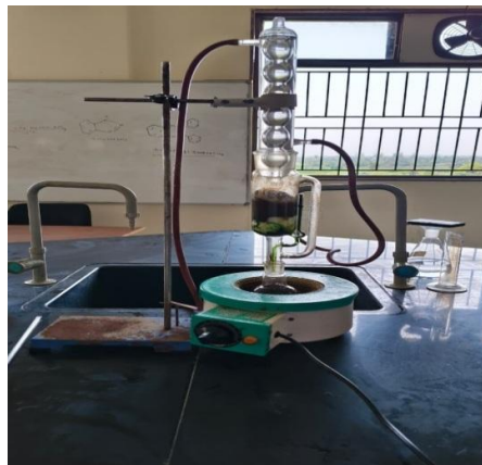
Fig. no.2 Soxhlet extraction apparatus
