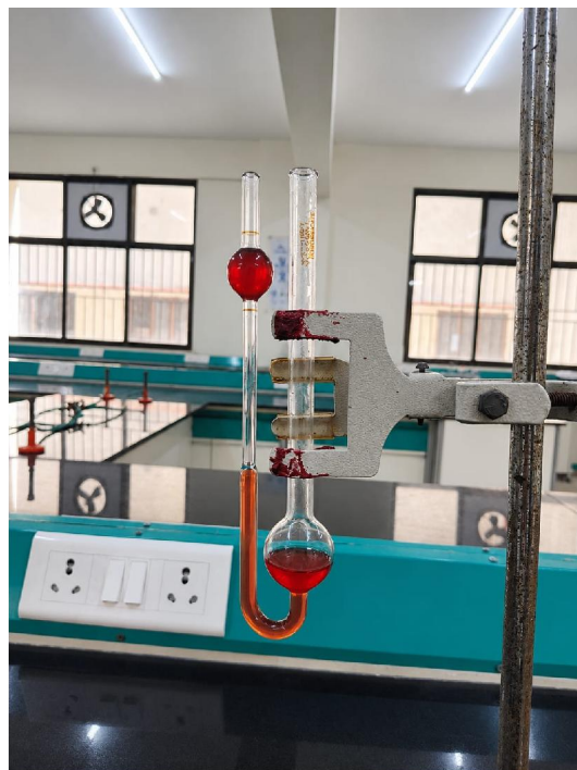
Fig. Ostwald's Viscometer Apparatus
