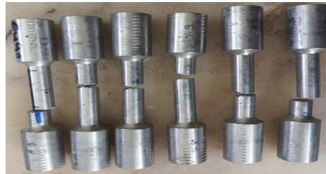
Fig. 4.5 Fractured Tensile testing specimens
