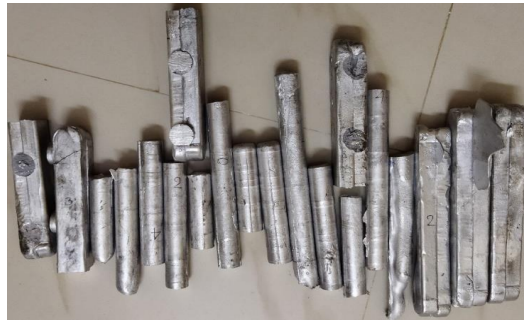
Fig. 3.5 Fabricated components through stir casting
