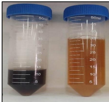
Fig 8:- Separation of silver nano particles
