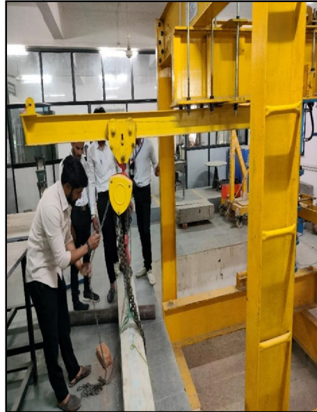
Fig 1: Beam Load Testing Setup
