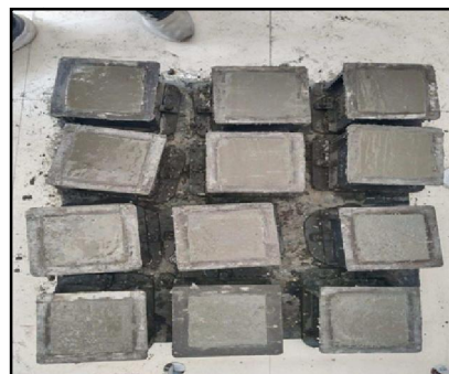
Fig 7: Concrete Cube Casting DOI: 10.48175/IJARSCT-35330
