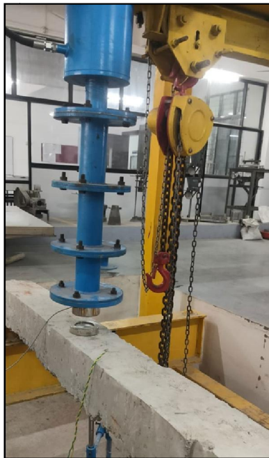
Fig 2: Hydraulic Jack Testing
