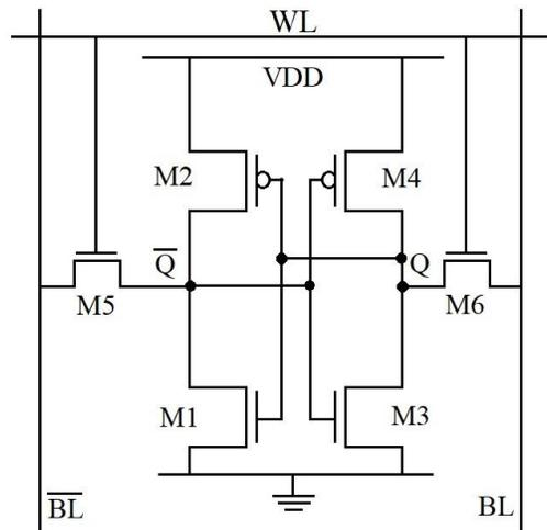
**Figure 1:** 6-Transistor Static Random Access Memory (SRAM)
