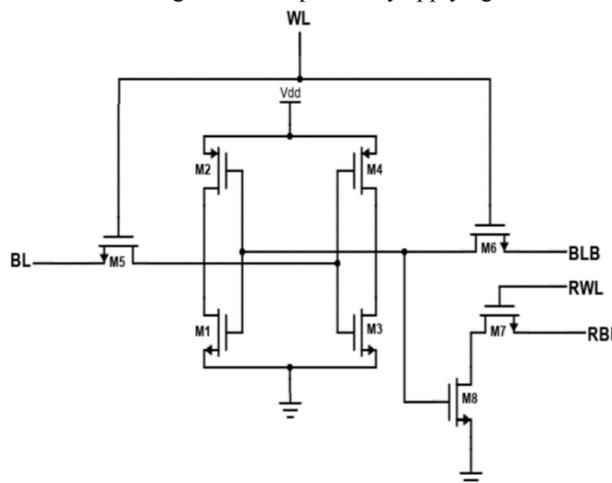
**Figure 4: 8T Conventional SRAM**
