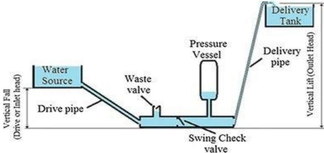
**Step 3:** As the pressure wave or spike moves back up the pipe, it creates a lower pressure situation (green arrows) at the waste valve. The spring-loaded check valve closes as the pressure drops, retaining the pressure in the pressure chamber.
