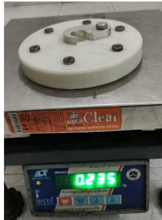
Figure 8: Weight of PLA jig plate with latch washer and bush
