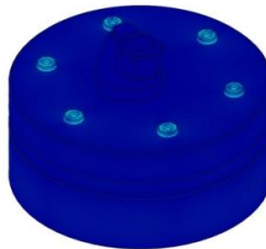
Figure 4: Stress Analysis of drill jig assembly
