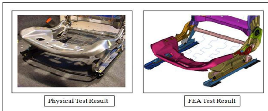
Figure 3 : Twisting of cushion pan
