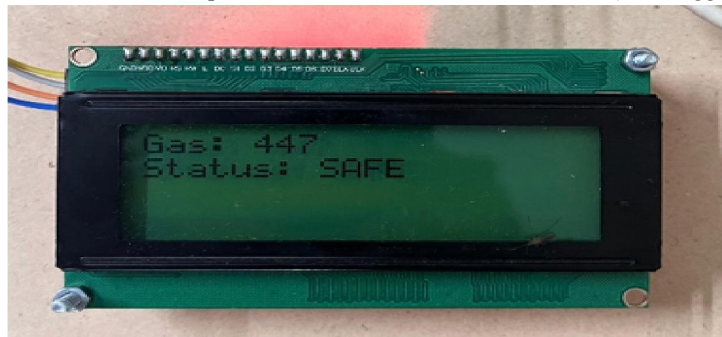
Fig. 9. LCD receiver output — Gas level: 447 ppm, Status: SAFE (normal condition).
