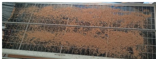
FIGURE VI SOLAR PANEL COVERED BY DUST AT 60%
