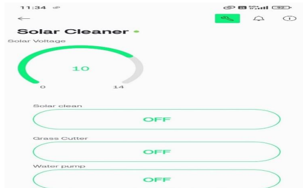
FIGURE VII SOLAR VOLTAGE WHEN SOLAR PANEL COVERED BY DUST AT 60%
