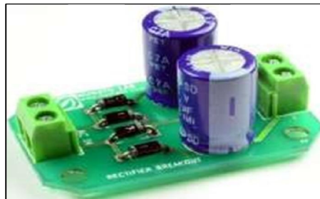
Fig 3: Bridge rectifier DOI: 10.48175/568
