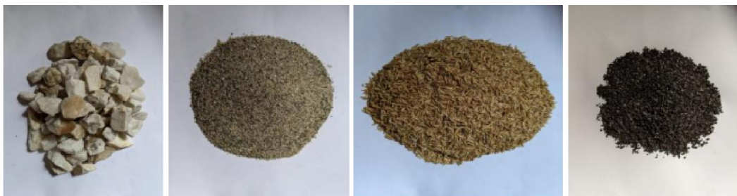
Fig. 2. Filter Materials (Pebbles, Sand, Corncob and Charcoal from left)
