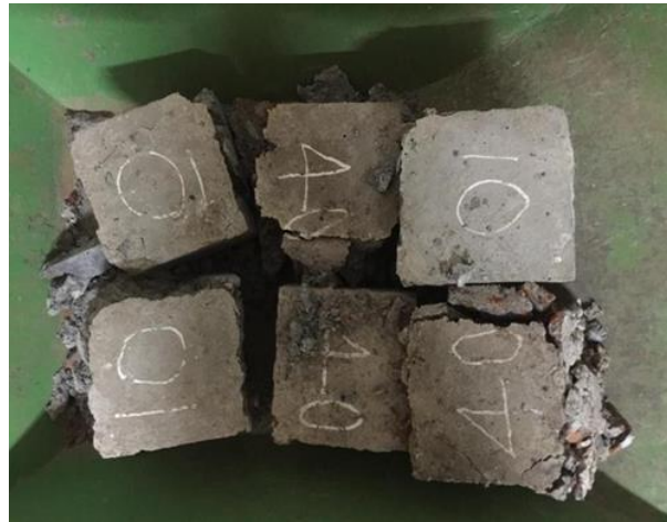
FIG. 2. CASTED CUBE AFTER REMOLDING
