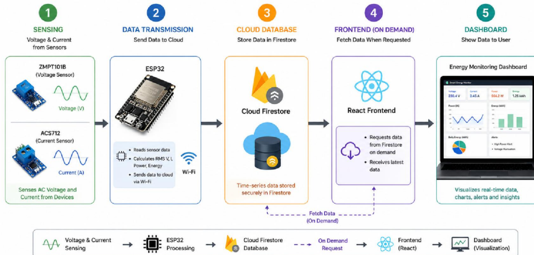
Fig. 1. Five-layer architecture of the Smart Energy Monitoring System spanning physical sensing, embedded processing, wireless communication, cloud services, and user-facing visualization.
