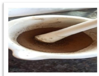
Fig 3. Formed Ferrite crushed in mortar and pestle to form fine ferrite powder
