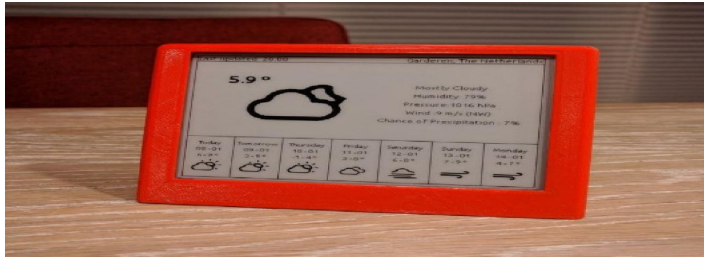
Fig 5.1 Final assembly and output of the 3D-printed enclosure with 4.2"EPD
