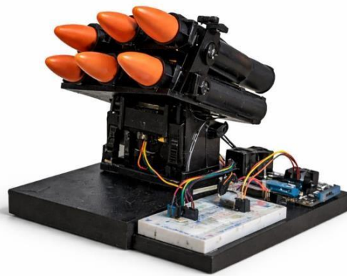
Fig. 3. Automatic Target Locking Missile Launcher System Model.
