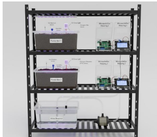
Fig. 2. IOT-powered vertical Farming in Stack Container
