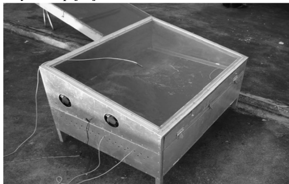
Fig. 4. Illustration of a cabinet-type solar dryer setup [76]
