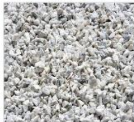
Stone aggregate is heated(160°-170° C) heated agg
