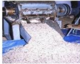
Plastic waste is shredded (2-4mm)
