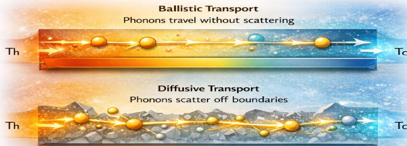
Figure 1: Schematic of Ballistic vs. Diffusive Heat Transport in Nanostructures
